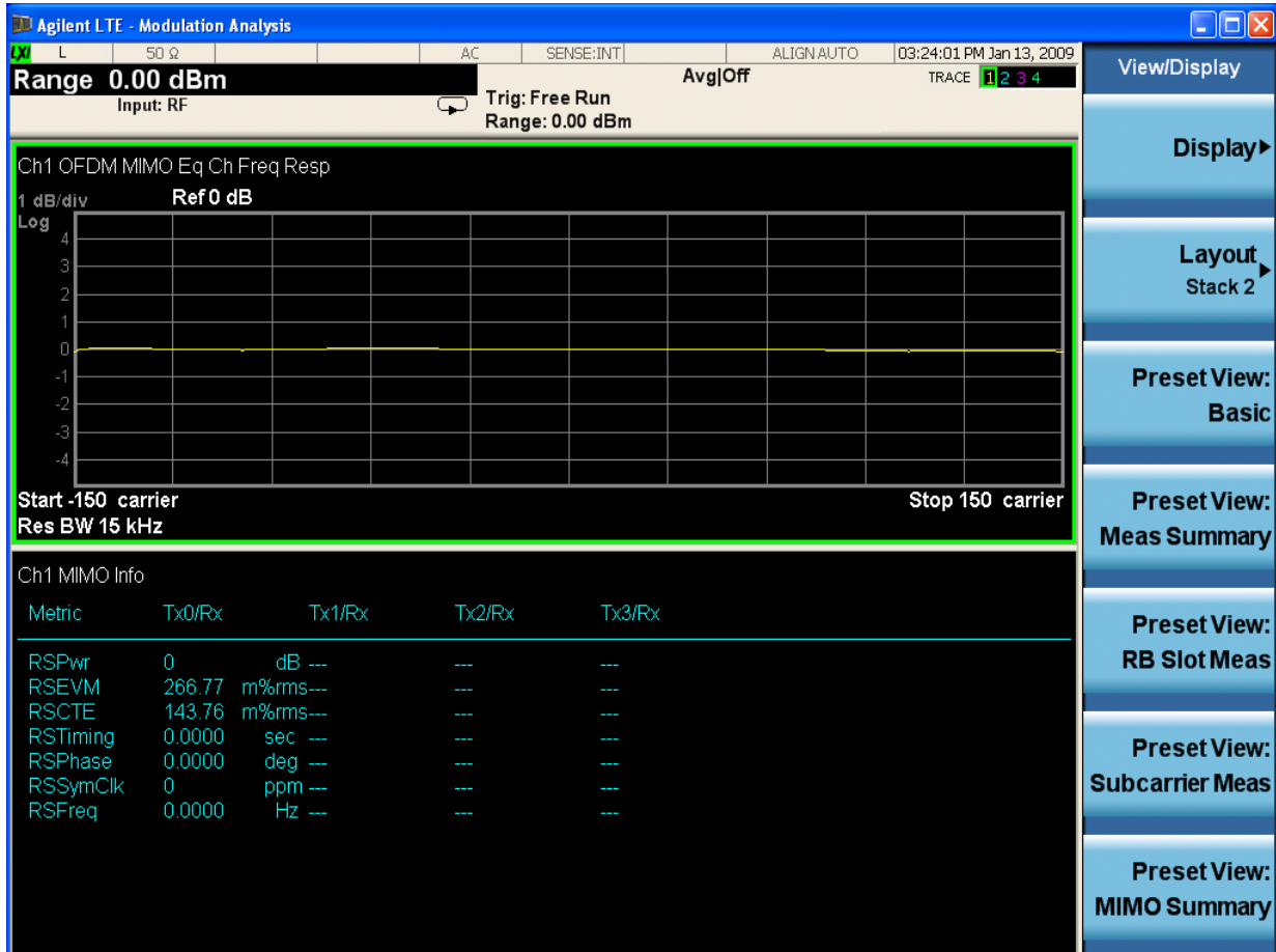
Figure 2-12 Modulation Analysis Measurement Result - MIMO Summary Preset View
